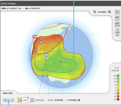
**PLOT REQUIRED DISH SIZE, C/I, C/N, C/(N+I), ΔT/T, OFF-AXIS EIRP OR PFD**
