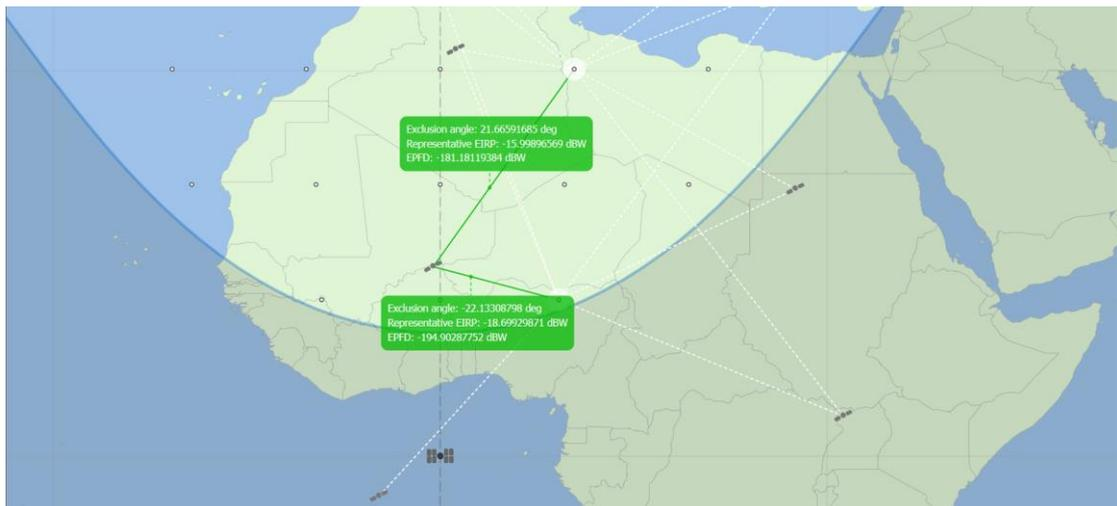
**Figure 18: Showing links between non-GSO satellites and Earth stations**
