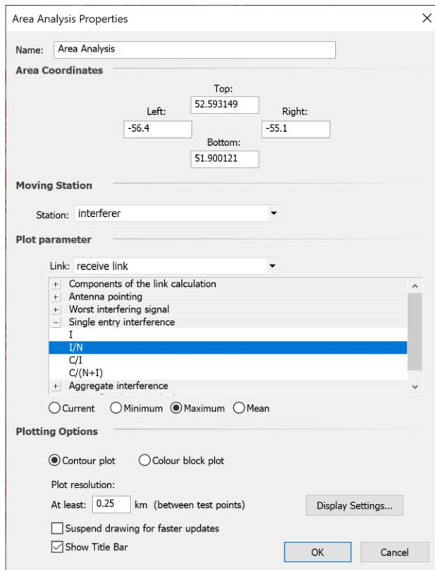
Selecting the Display Settings button in this window allows us to configure the contour. This is set to -19 dB and coloured red. That is, any pixels coloured red or enveloped by the red contour in the area analysis are locations where the presence of the IMT base station leads to excess interference at the receiver.
