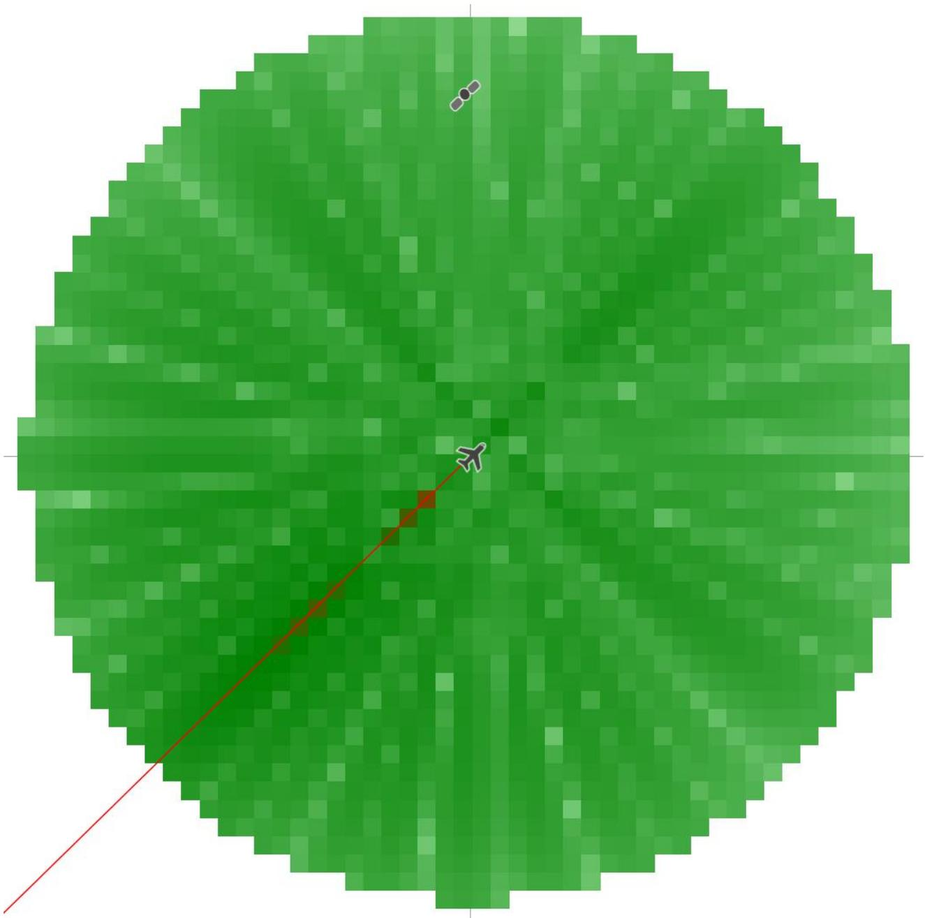
The peaks and troughs of the M.2101 gain pattern can be seen around the A-ESIM, and a zone of higher PFD in the direction of transmission.
