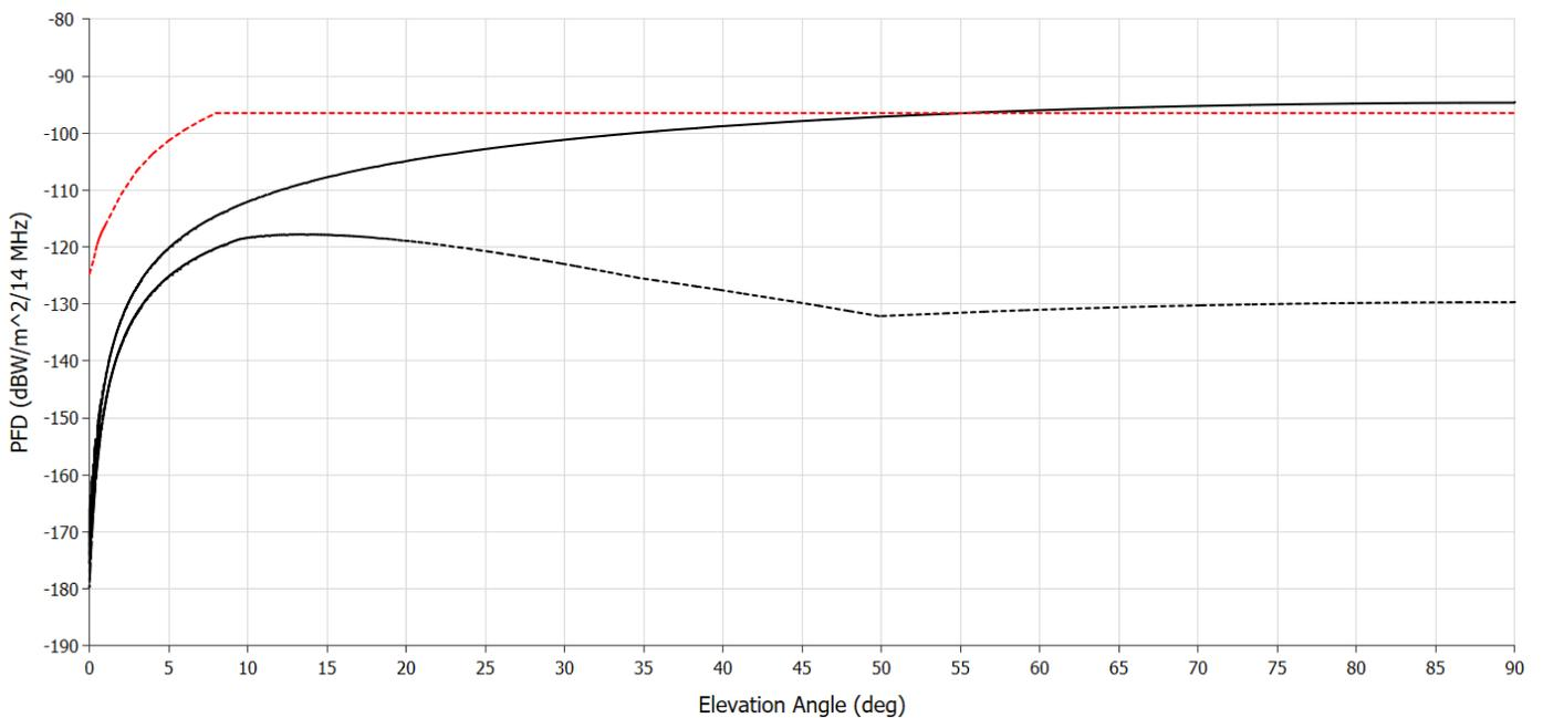
It can be seen that the Resolution 169 PFD limits are exceeded at high elevation angles in the case where no fuselage loss is included (solid line) but met for all elevation angles when fuselage loss is included (dashed line).
