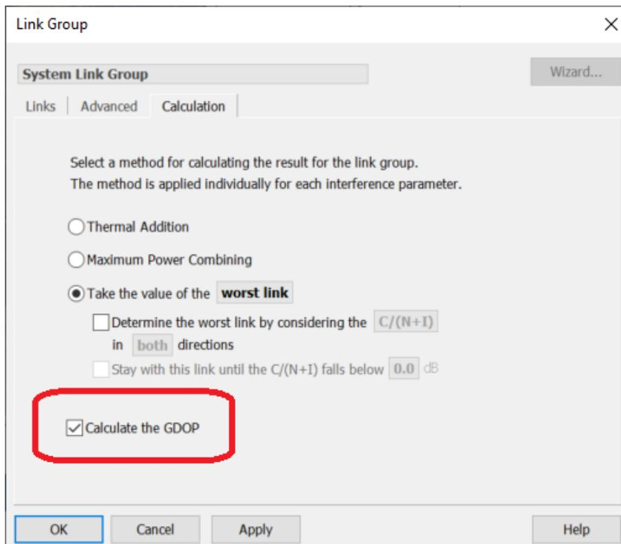
When selected, the GDOP is calculated over all the Links in the Link Group. For example, in this case, it would be calculated for 5 Links:
