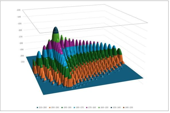
ITU-R M.2101 for beamforming antennas, where the peak gain and sidelobes changes as it is steered. An example of the PFD from a single pointing direction using an antenna with gain pattern from M.2101 is shown below:
