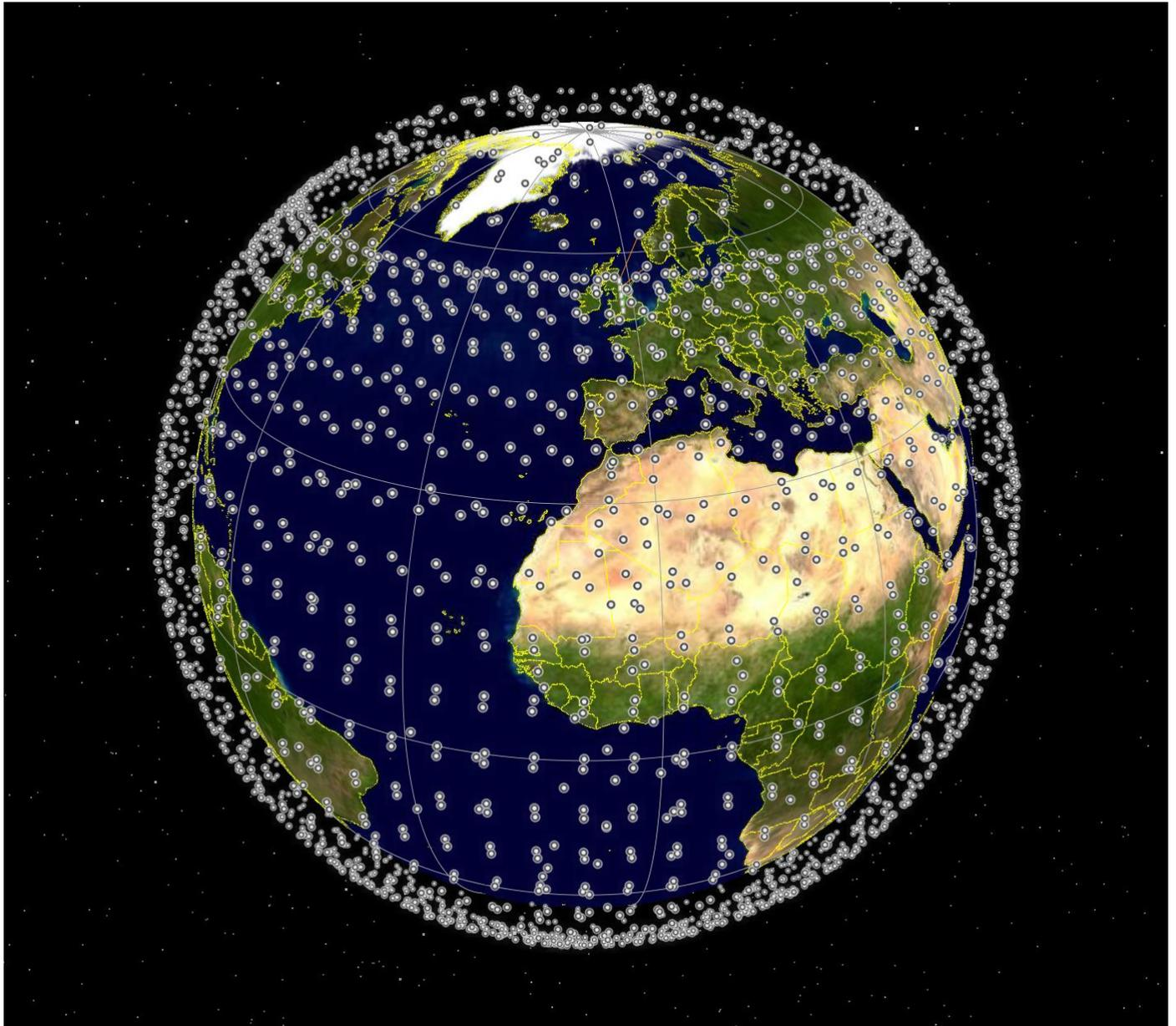
This constellation, based upon a SpaceX filing, contains over 4,400 satellites at an altitude between 550 and 570 km, most at an inclination angle of around 53 degrees but with some polar planes.
