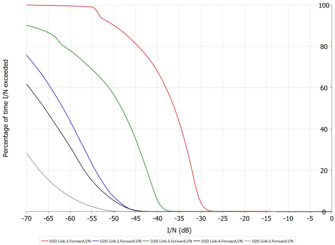
It can be seen that, in general, interference levels are low when the locations are separated by 1° of latitude (around 111.1 km). Interference into the D2D system decreased, the greater the separation distance to the mobile networks.
