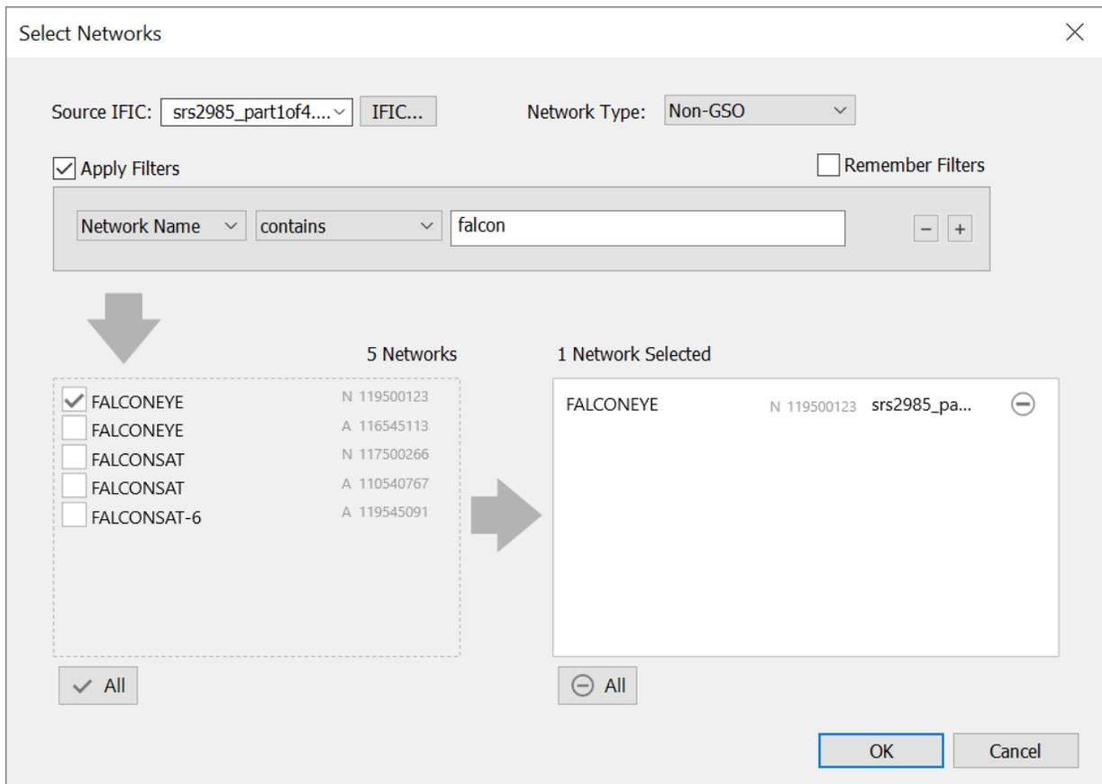
When in the internal database, a non-GSO system can then be considered during an IFIC check, in particular, to check for frequency overlap with other non-GSO systems.
