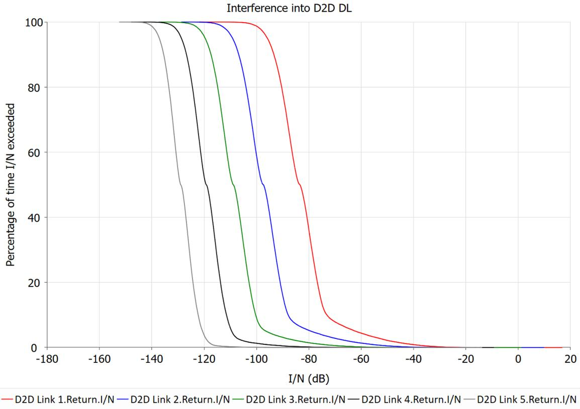
It can be seen that, in general, interference levels are low when the locations are separated by 1° of latitude (around 111.1 km). Interference into the D2D system decreased, the greater the separation distance to the mobile networks.
