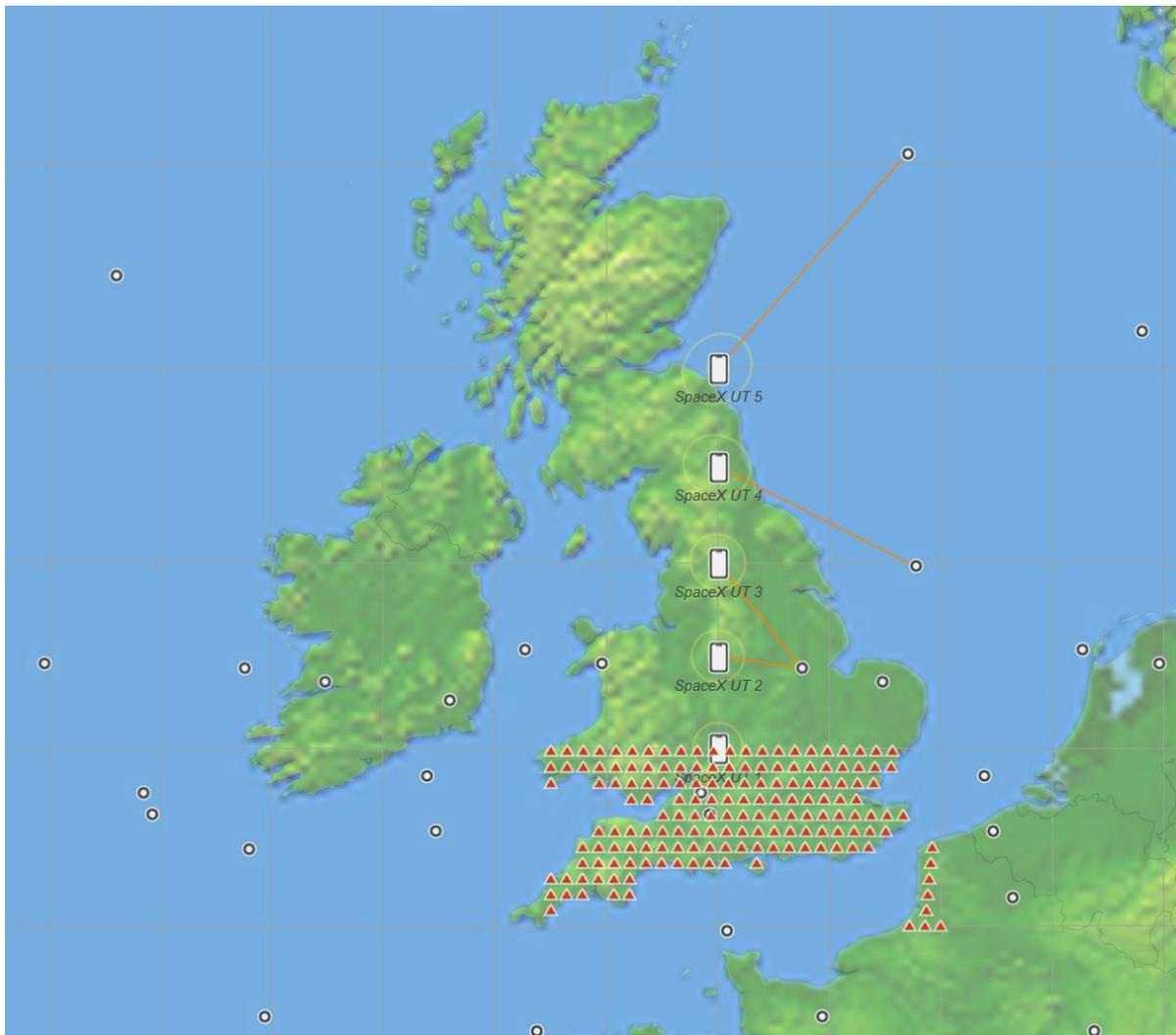
Here, the service area wizard has been used to deploy a grid of 162 stations with separation 20 km across the land mass of England and Wales south of the lowest latitude D2D UE. To avoid the first of the D2D UEs being co-located with some of the terrestrial mobile stations, the array of D2D UEs was moved north  $1^\circ$ .
