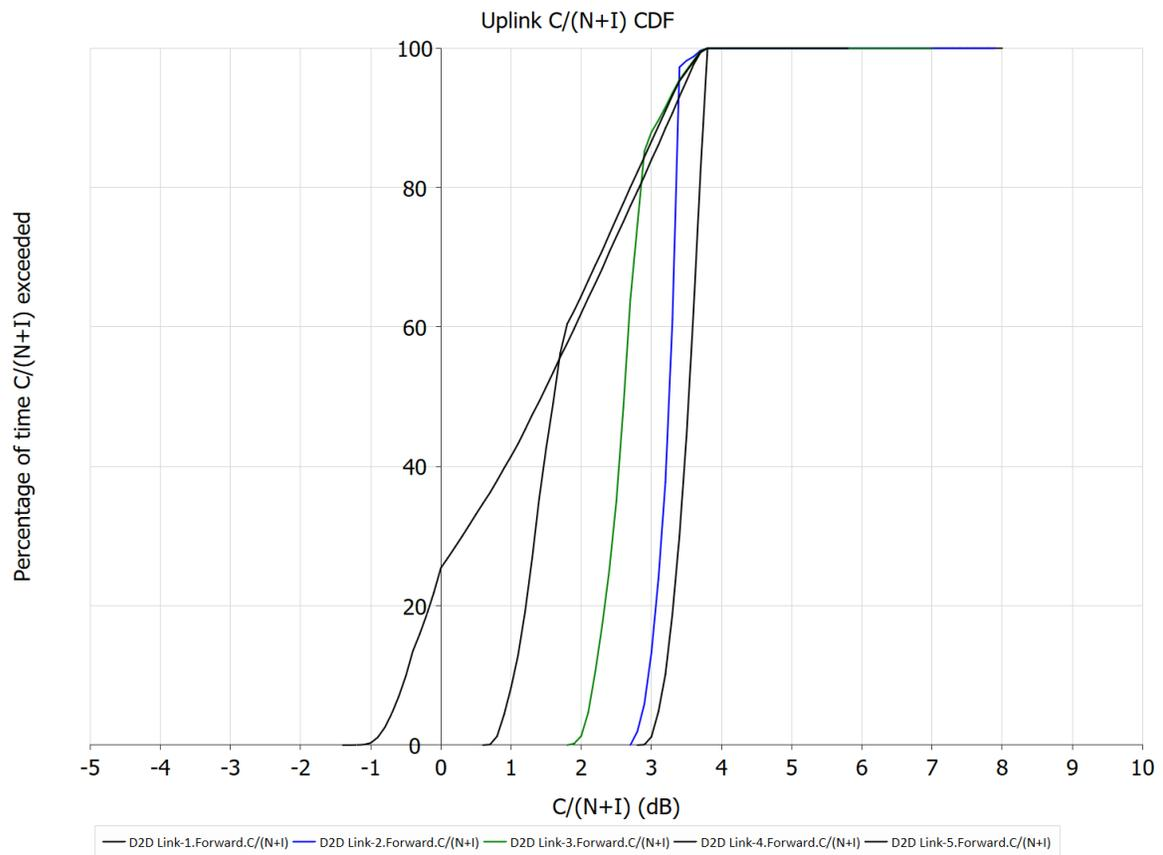
Minor degradations in the C/N due to interference can be seen in the figures above and the table of derived values below:
