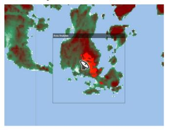
It can be seen that the impact of considering terrain is to significantly reduce the size of the contour.
