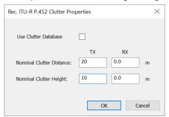
Note that the receive end could be anywhere within the Area Analysis and hence there could be a range of distance to clutter and height of clutter. If a land use database is available it could be used to determine the nominal clutter distance and height to use at the transmit and/or receive ends.
