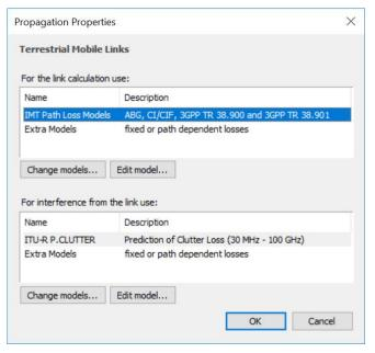
The extra loss is simply zero while the P.Clutter is configured to be the statistical model considering a random loss at the transmit side, as per the following:
