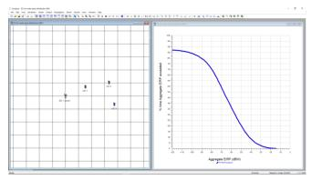
Note that the AEIRP CDF does not go all the way up to 100%: this is because the likelihood that each link is active is 50% and hence not active 50%. The probability that all three links are not active is therefore  $(1/2)^3$  or 12.5%. Hence the time that at least one link is active is 87.5%.
