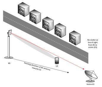
In the first case there is clutter loss between the BS and the ES and at 26 GHz this is likely to represent a significant attenuation of the interfering signal.
